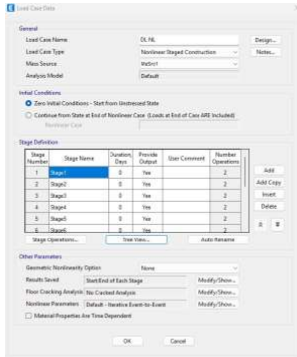
Figure 3. Load Case Nonlinier Stage Construction
